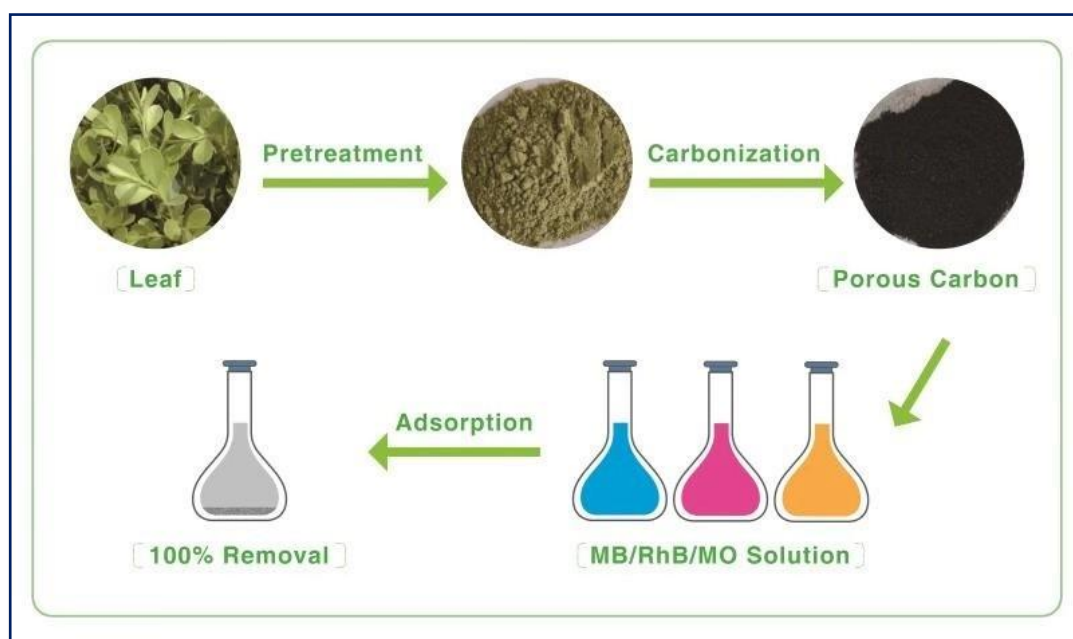
Fig. 4. Schematic representation of the preparation and application of porous carbons on dyes MB, RhB and MO from wastewater [52].
